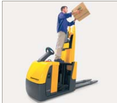
Order picking from second racking level with raised stand-on platform
