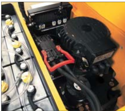
Drive and lift motor with AC technology
