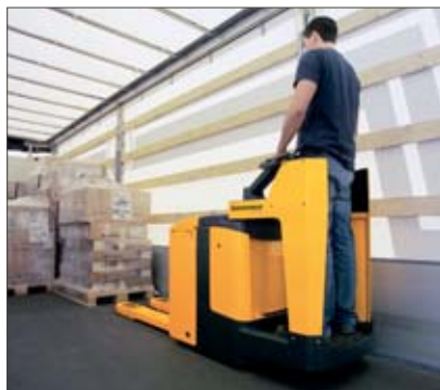
Protected operator workplace with fixed stand-on platform
